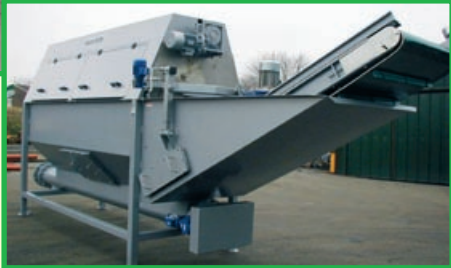
Barrel washer with sludge auger in base tank for automatic waste removal
