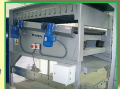
Air jack system to lower roller bed making servicing & cleaning easy and safe for the operator.
