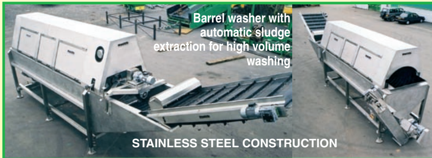
1mtr long brush mounted in out feed of barrel
