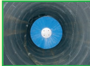
1mtr long brush mounted in out feed of barrel
